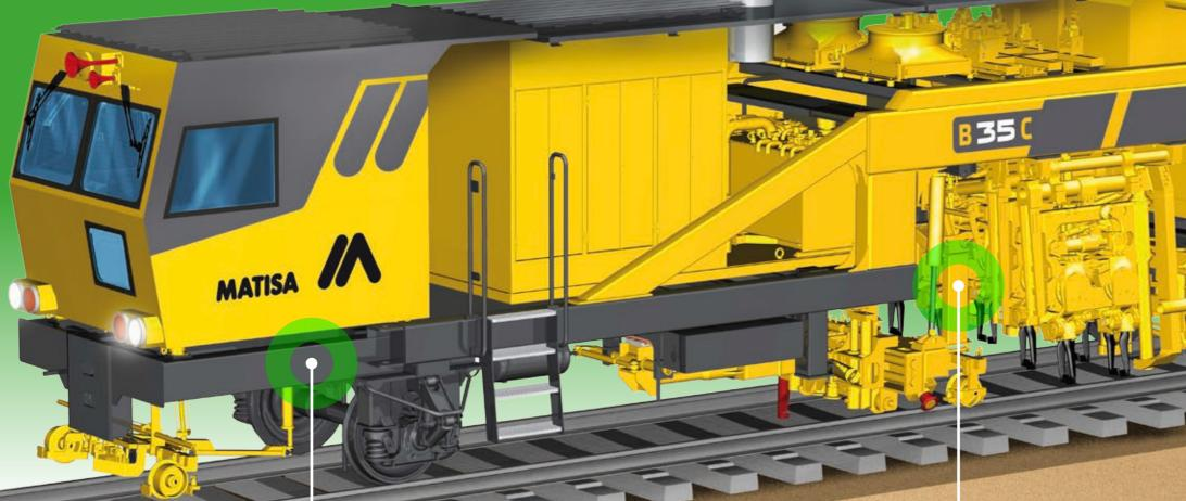
This machine has two air-conditioned cabins fitted with working and driving posts.
