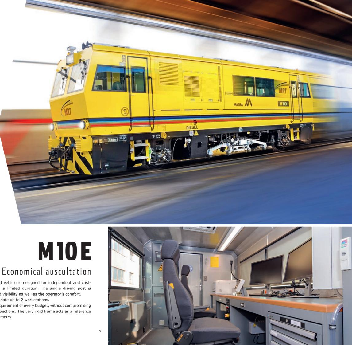
This small self-propelled vehicle is designed for independent and costefficient inspections for a limited duration. The single driving post is raised and ensures good visibility as well as the operator's comfort. The cabin can accommodate up to 2 workstations.
