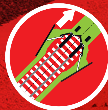
Space filling, transfer of excess from center outwards and brushing
